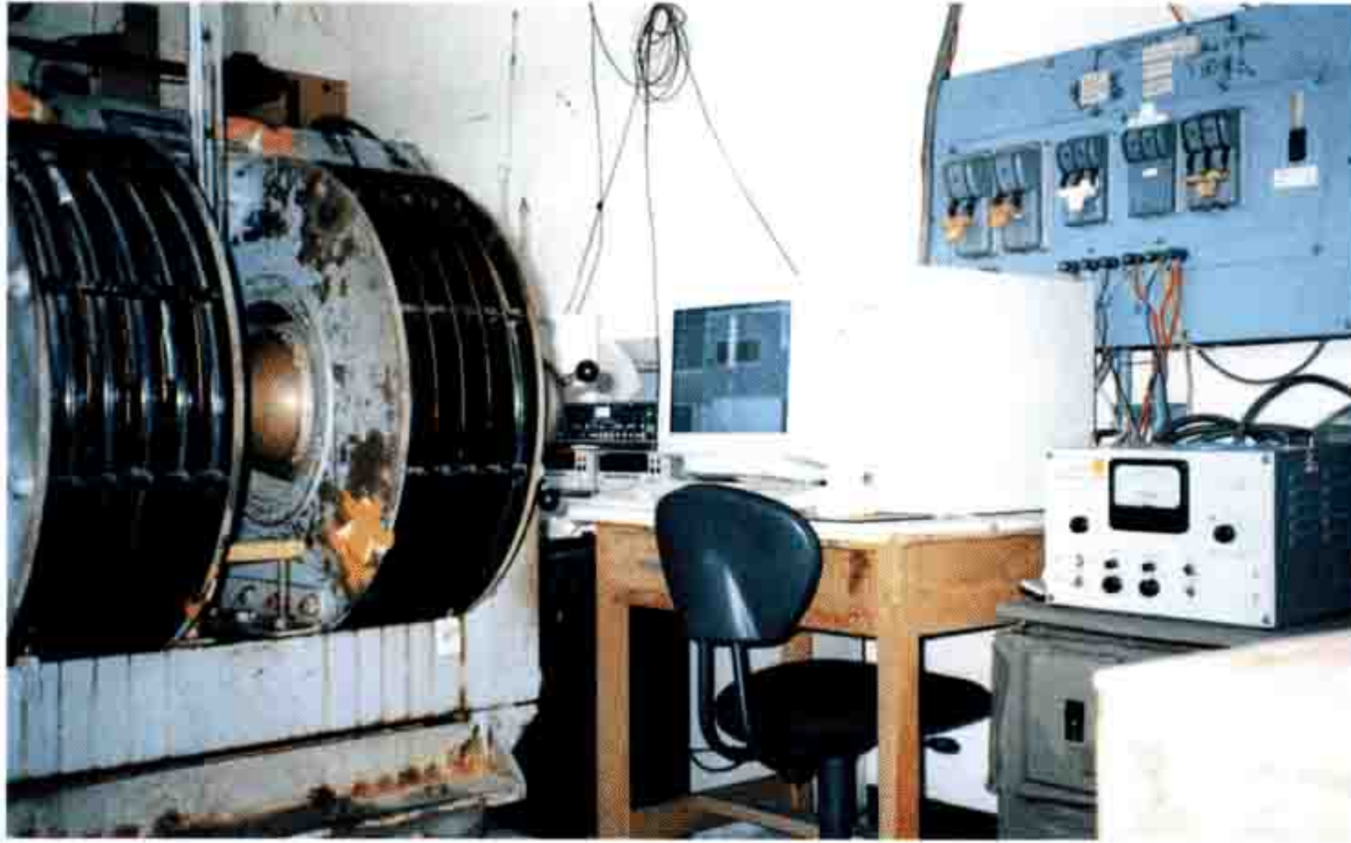
Water-cooled magnet (applied field H < 1.5T ) and equipment measuring Magnetic properties. (ac-susceptibility, magnetstriction etc.)
