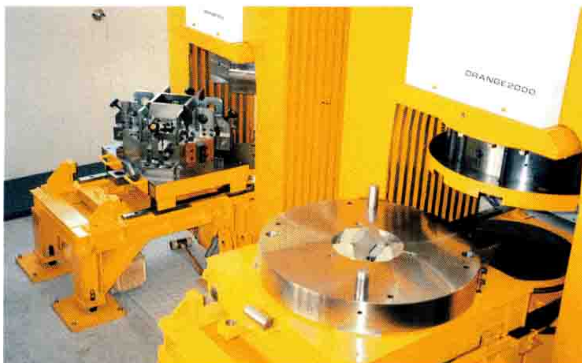
Multianvil apparatus (ORange-2000 and ORange-1000) at the Ultra-High Pressure Laboratory. These apparatus can produce pressures to 40 GPa and temperatures exceeding 2000°C, and are used to explore the constitution and composition of the Earth's deep interior.
